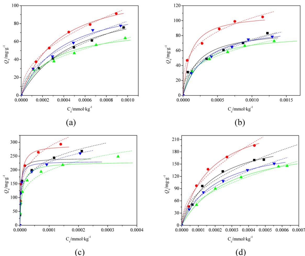
**Figure 5.** Adsorption isotherms for berberine hydrochloride (a), ligustrazine hydrochloride (b), colchicine (c), and matrine (d) on different resins at 30 °C: ■, HPD100B; ●, HPD300; ▲, AB-8; ▼, HPD722; —, Langmuire; ---, Freundlich.
