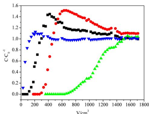
**Figure 6.** Dynamic adsorption breakthrough curves for an alkaloid mixture solution on HPD300 resin: ■, berberine hydrochloride; ●, ligustrazine hydrochloride; ▲, colchicine; ▼, matrine.
