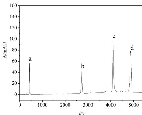
**Figure 2.** A HPLC profile of an alkaloid mixture sample of matrine (a), ligustrazine hydrochloride (b), berberine hydrochloride (c), and colchicine (d).
