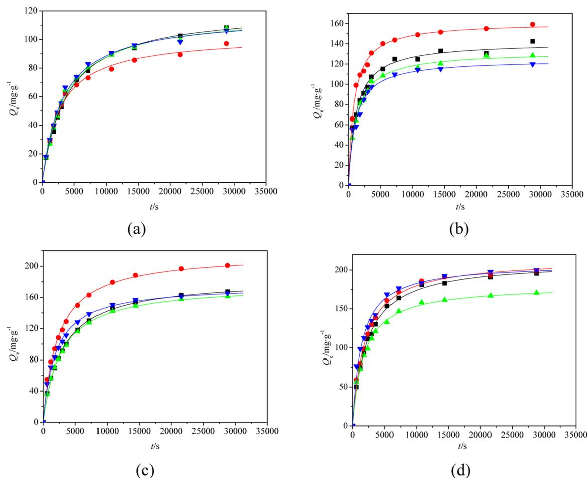
**Figure 4.** Adsorption kinetic curves for berberine hydrochloride (a), ligustrazine hydrochloride (b), colchicine (c), and matrine (d) on different resins at 30 °C: ■, HPD100B; ●, HPD300; ▲, AB-8; ▼, HPD722; —, pseudo-second-order.
